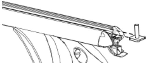
End cap can be opened to remove the rubber strip & insert T-Bolts for ease of adding accessories. You will need to cut the rubber strip to reinsert around the T-Bolts, and maintain the weatherproofing of the roof bars.
